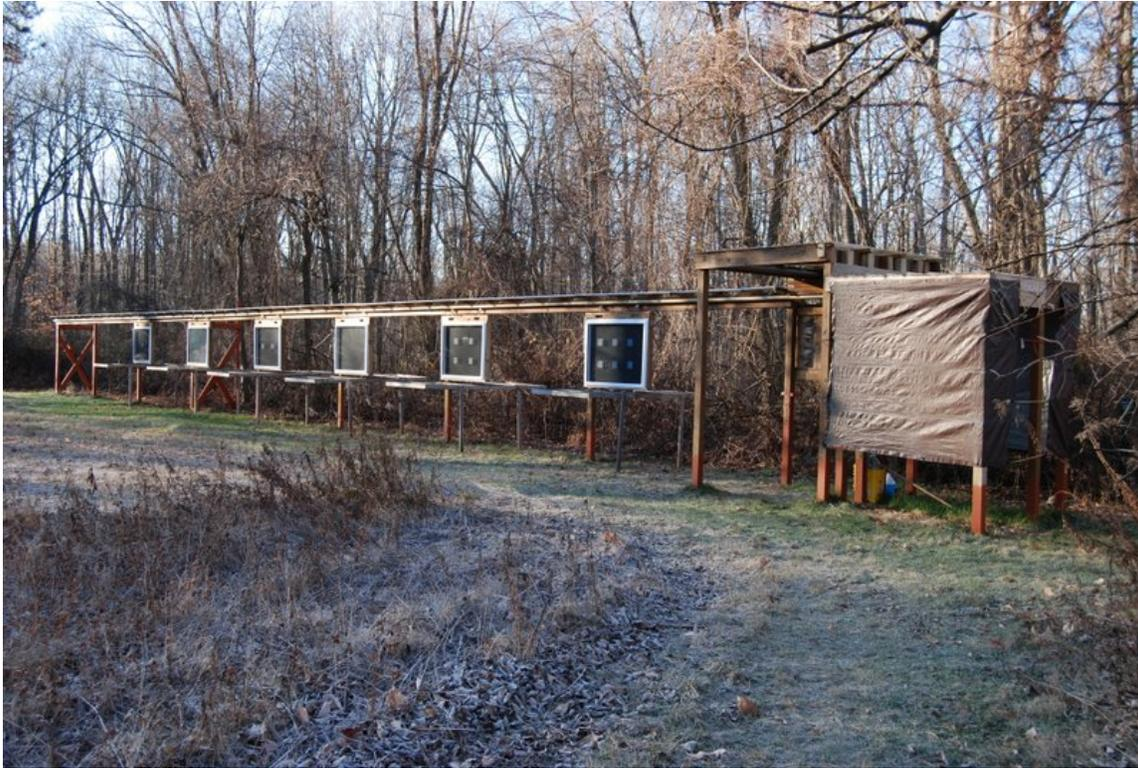
Figure 1. Wooden-framed experimental structure with treatments (control and varying numbers of BEV film elements) in rural Henningsville, Berks County, Pennsylvania, USA); photographed Sunday 3 January 2016 by P. G. Saenger.
