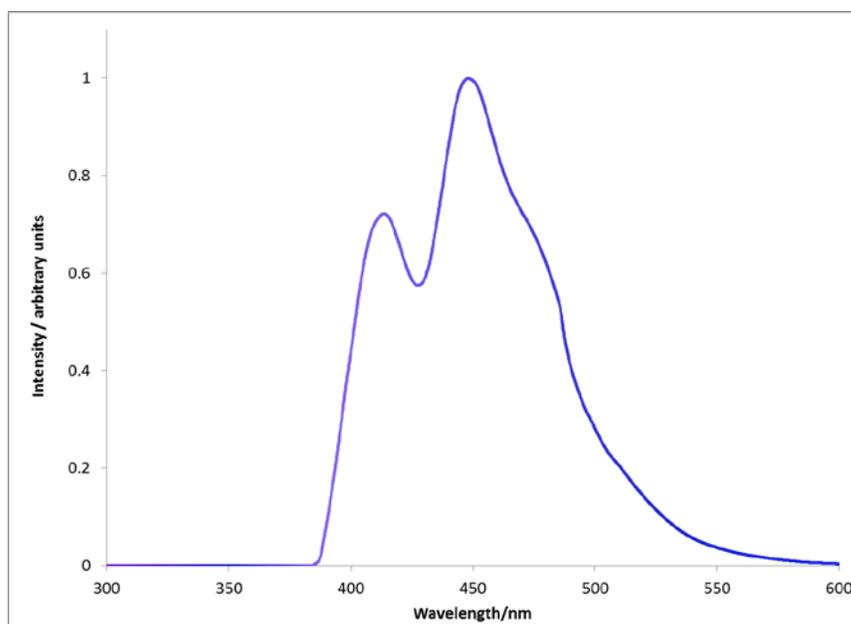
Figure 5. The spectrum that results from 410 nm light striking glass with Bird's Eye View film affixed to the back. The peak at 410 nm is the result of incident light reflecting off the surface of the glass and the peak at 450 nm is the result of light being emitted by the Bird's Eye View film. Legend and graph by Steven G. Mayer, Professor of Chemistry, University of Portland, Portland, Oregon.
