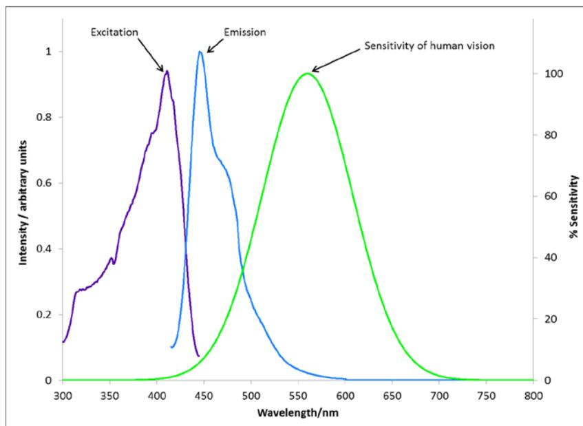
Figure 4. Spectroscopic data showing the range of light absorbed (excitation) and the light emitted (emission) by the Bird's Eye View film. The green curve shows the approximate spectral response of the human eye. Legend and graph by Steven G. Mayer, Professor of Chemistry, University of Portland, Portland, Oregon.
